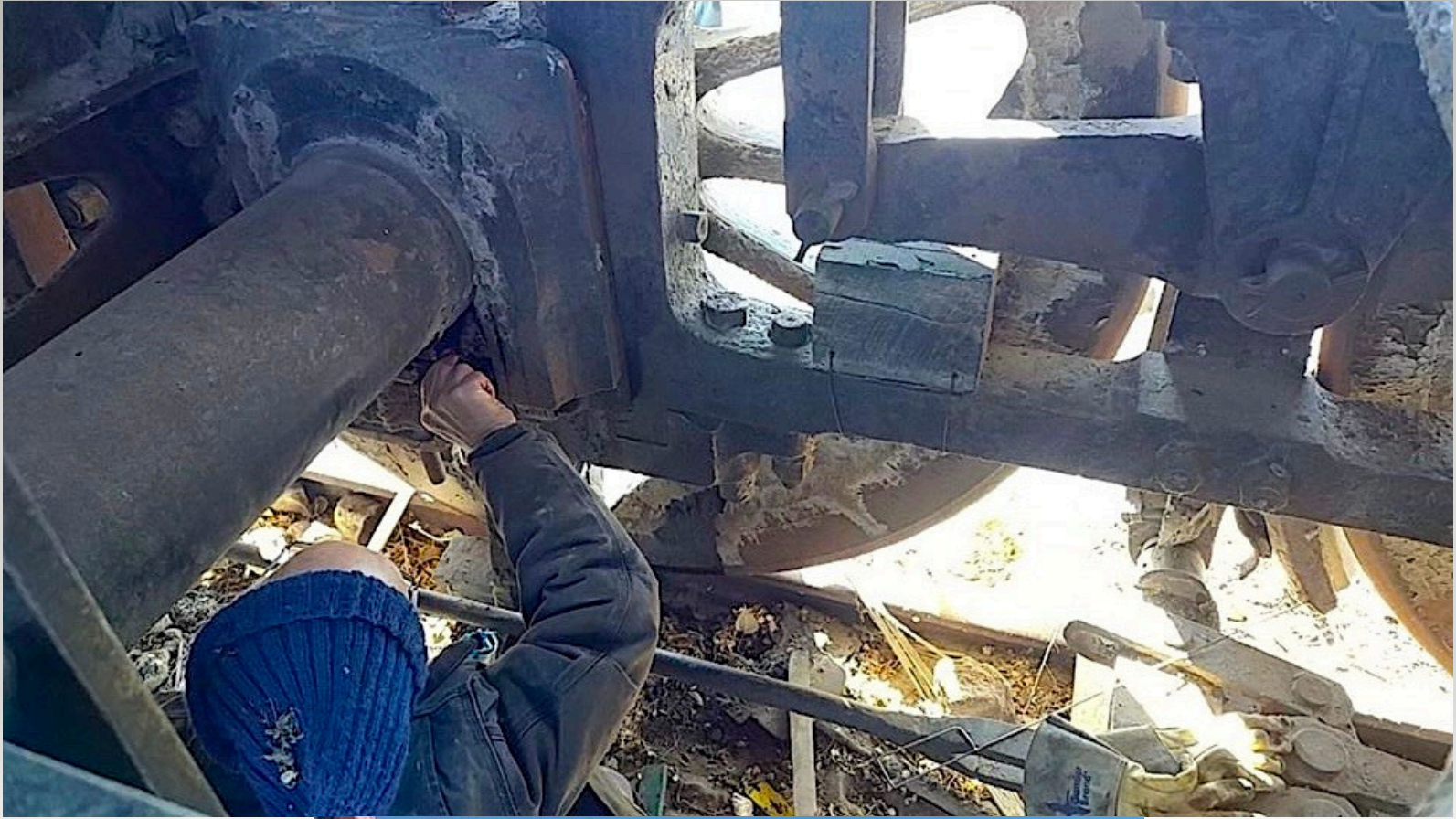
Al Broadfoot inspecting the grease cellars
